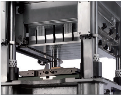
Sonotrode table with flat sealing area
