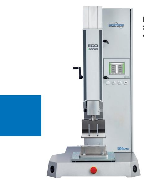
ECO iSONIC Standard machine with pneumatic drive
