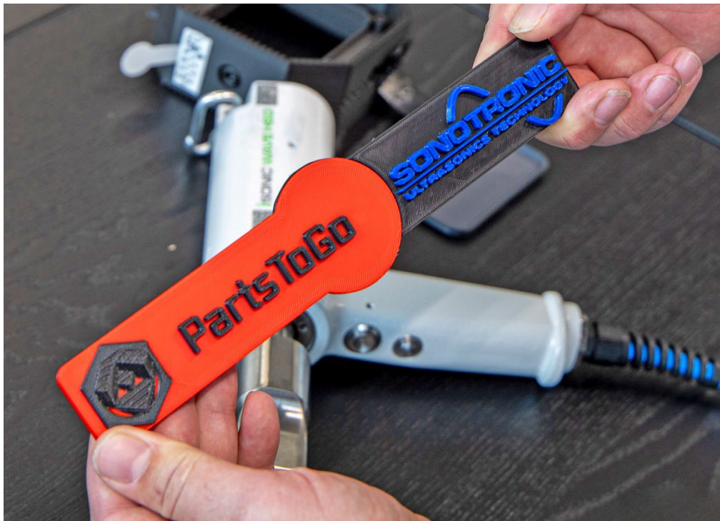
Caption: The result of the ultrasonic process: The two 3D-printed plastic parts are precisely and completely welded into a stable component without any additives.
