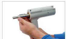
Our new DNP iSONIC handheld welding device has an ergonomic design and a sturdy cast aluminium housing featuring a quick-change mechanism for the sonotrode. Thanks to the integrated sonotrode cooling system, DNP iSONIC is also suitable for continuous use, e.g. for small series, manual workstations, repairs or finishing tasks.
