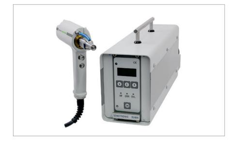
Our new iSONIC WAVE HSG handheld welding device has an ergonomic design and a sturdy cast aluminium housing featuring a quick-change mechanism for the sonotrode. Thanks to the integrated sonotrode cooling system, iSONIC WAVE HSG is also suitable for continuous use, e.g. for small series, manual workstations, repairs or finishing tasks.
