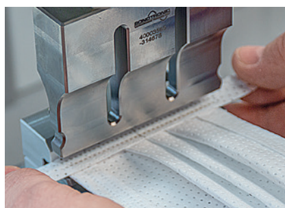
5. The non-woven are fastened by vertical ultrasonic welding of side seams 3 and 4.
