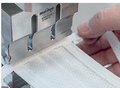
4. Placing of non-woven, used for the fixation on the head, at the short side.
