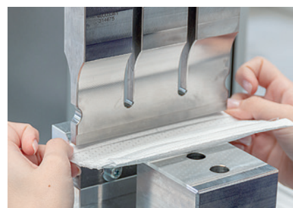
3. Horizontal ultrasonic welding of cross seams 1 and 2. The nose band is slid in manually (no illustration).
