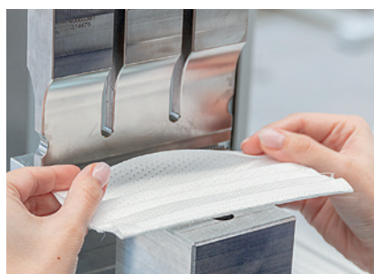
2. Manual folding of the non-woven edge before ultrasonic welding.
